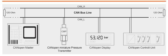
The use of CANopen bus protocol for pressure transmitters allows easier cabling, configuration via bus software, regular condition monitoring of the sensor itself and measurement of pressure and temperature with
