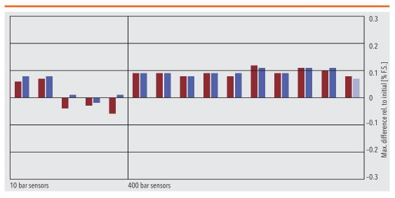
Extreme tests with load changes show that the sensors from Trafag are still stable and usually deviate by less than 0.1 % from the initial value after 10 or 20 million cycles and twice the rated pressure.
